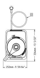
Electric Supply voltage: 220-240 V/1N ph/50/60 Hz Electrical power, max: 0.75 kW 0.75 kW **Total Watts:** Capacity: Performance (up to): 0 kg/Cycle Capacity: 3.6 litres Key Information: External dimensions, Width: 252 mm External dimensions, 334 mm Depth: External dimensions, Height: 476 mm **Shipping weight:** 19 kg Meat mincing capacity: 0 kg Mayonnaise preparation 0 kg capacity: Pastry preparation capacity: 0 kg
